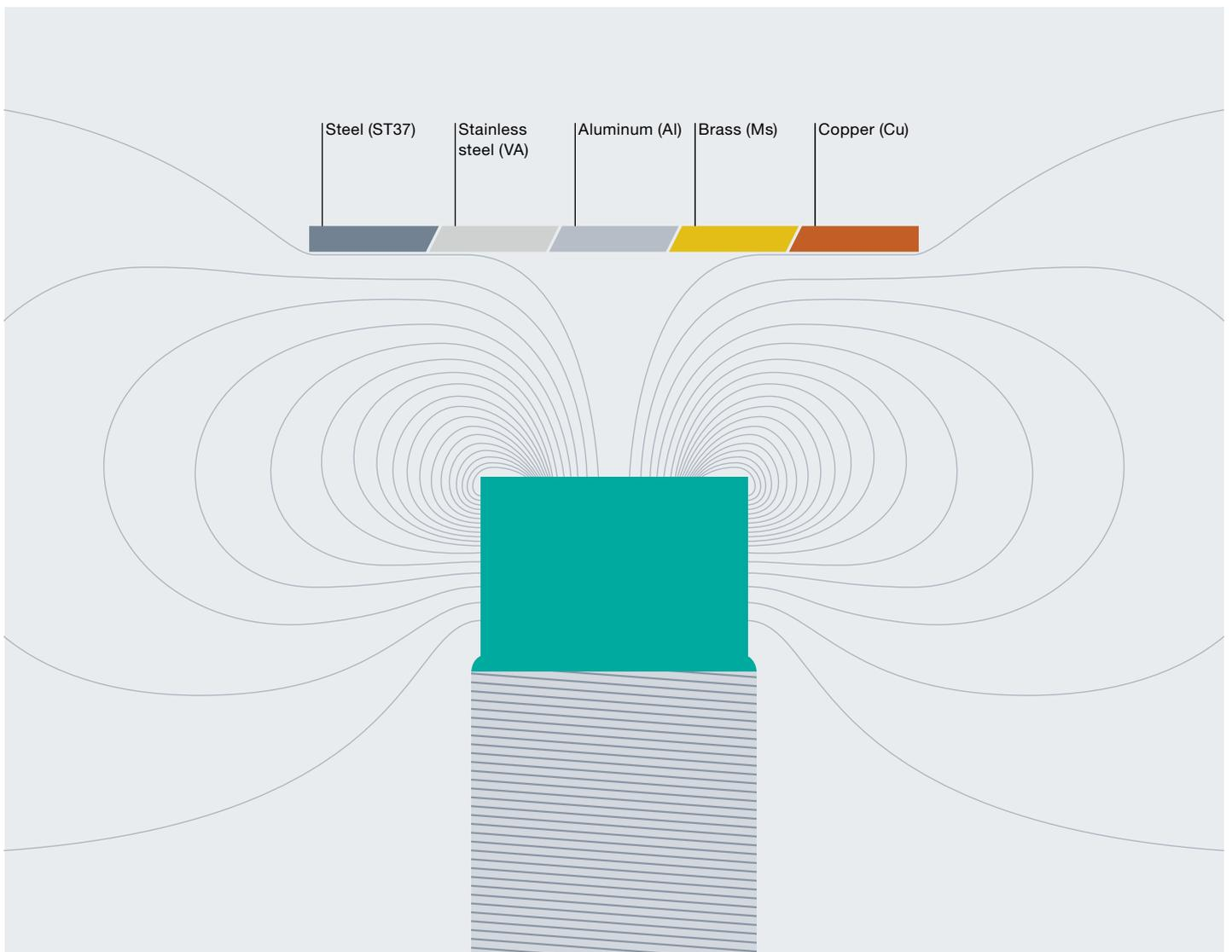
Non-flush reduction factor 1 sensors offer high and identical sensing ranges for all metals.
