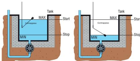
This function is achieved by connecting the black and brown float terminals. The level regulator contact closes the upper circuit at maximum level and opens the circuit when the float reaches the lower minimum level. The MIN and MAX levels can be adjusted by varying the distance between counterweight and float.
