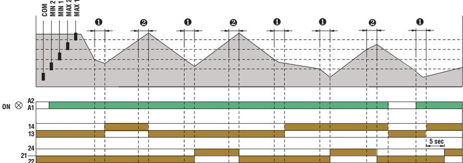
Filling tank and draining well function + alarm
