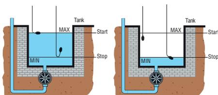
This function uses two floats and is achieved by connecting the black and brown float terminals. The MIN and MAX levels can be adjusted by varying the position of the floats.
