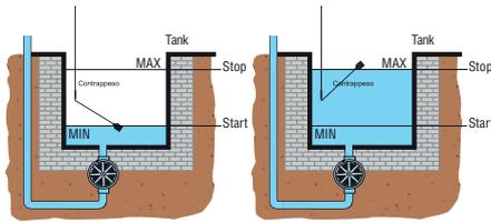
This function is achieved by connecting the black and blue float terminals. The level regulator contact closes the lower circuit at minimum level and opens the circuit when the float reaches the upper maximum level. The MIN and MAX levels can be adjusted by varying the distance between counterweight and float.
