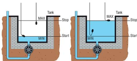
This function uses two floats and is achieved by connecting the black and blue float terminals. The MIN and MAX levels can be adjusted by varying the position of the floats.
