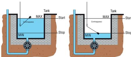
This function is achieved by connecting the black and brown float terminals. The level regulator contact closes the upper circuit at maximum level and opens the circuit when the float reaches the lower minimum level. The MIN and MAX levels can be adjusted by varying the distance between counterweight and float.
