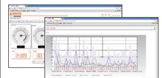
It is a server-multiclient system based on MS SQL RDBMS with web-browser interface. Simultaneous management of different communication channels with independent configuration (protocols, speed rate, RS232, RS485, Ethernet, modem) is possible. Live page view, data log tables, charts and alarms are available.
