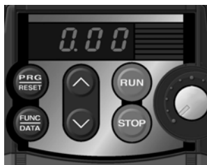
Figure 4.2 Display of the LED Monitor after Power-on
